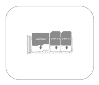
3. Hold your device face up, and then slide the tray all the way into t he slot in the direction as indicated by the arrow.
