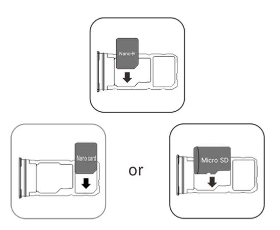
3. With the touch screen facing up, follow the direction of the arrow to install the tray (with Nano card ) into the phone.
