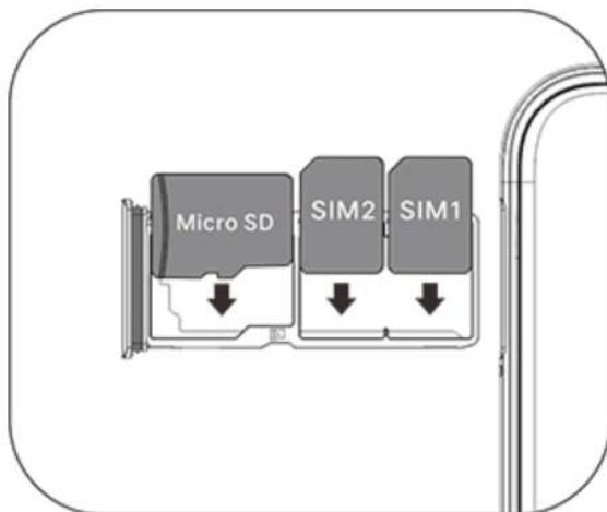
3. Touch screen facing up, follow the direction of the arrow to install the tray (with Nano card or Micro SD) into the phone.
