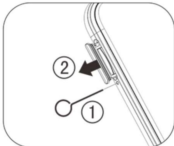
2. Make the metal face of the Nano card (SIM1/SIM2) or Micro SD card face downward, with the oblique angle corresponding to that of card tray. Put the Nano card (SIM1/SIM2) or Micro SD card into the card slot according to the direction indicated by arrows of the diagram.
